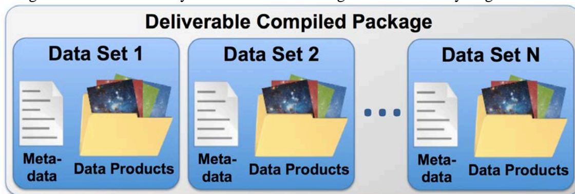
Figure 3 Compiled package delivered to user, generated from a single query of the coronagraph PSF library. For each of N exposures that match the query criteria, the compiled package contains a corresponding data set. Each data set contains metadata and a bundle of data products, which contains the exposure itself and any additional pipeline data products requested.
